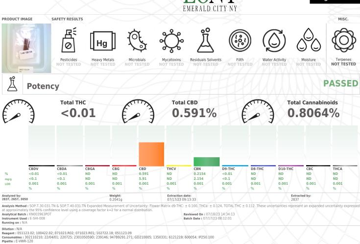
Full spectrum cannabinoid analysis utilizing High Performance Liquid Chromatography with UV/PDA detection (HPLC-UV/PDA). All cannabinoids have an LOQ of 0.01%
